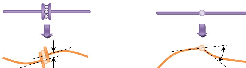
Figure 2.39: Schematics of deformed shape in the neighborhood of the shear and moment releases
